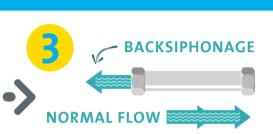
Because of the suction created by the drop of pressure in the public water system's main, the water in the pool will be sucked back through the hose pipe into your internal plumbing, and then out into the public's drinking water system
